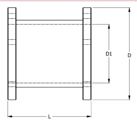
$$\begin{array}{lll} D & = 110 \\ D1 & = 80 \\ L & = 100 \\ Torque (N m) = 160 \end{array}$$
